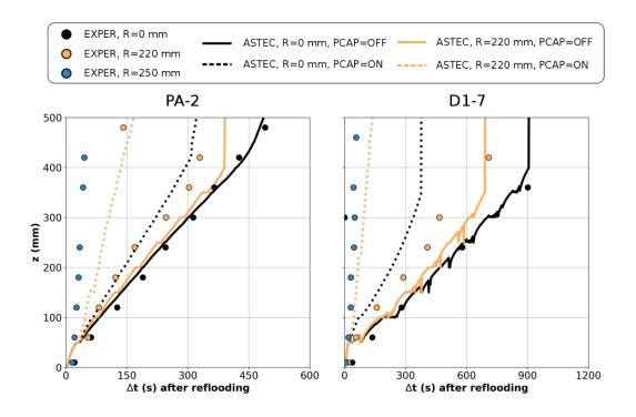
Figure 11: Predicted vs. Experimental evolution of the quench front for the tests PA-2 and D1-7 (see Table 1) with and without the capillarity correction.
