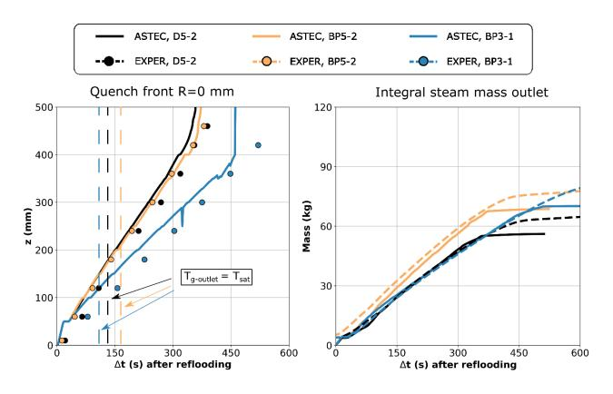
Figure 8: Predicted vs. Experimental evolution of the quench front evolution at R=0 mm and cumulated mass of steam at the outlet for the tests D5-2 and BP5-2 (5 bar, 700°C, 5 m/h) and BP3-1 (3 bar, 700 °C, 5 m/h).
