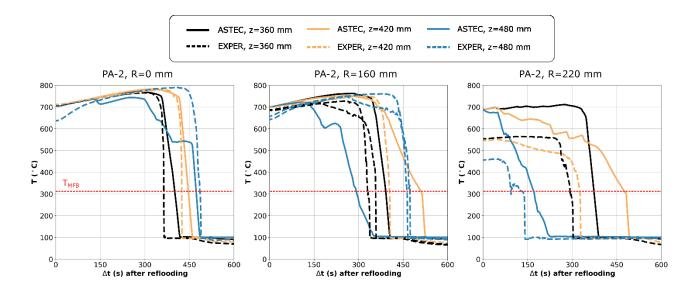
Figure 17: Evolution of computational (without capillarity) and experimental debris temperatures at selected radial and axial locations for the test PA-2. Red horizontal line represents the minimum film boiling temperature. Two experimental lines of the same kind indicate measurements at two different azimuthal positions.
