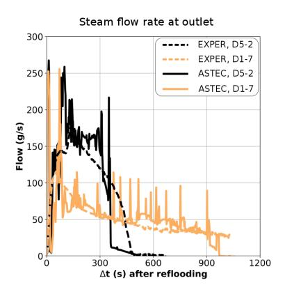
Figure 7: Predicted vs. Experimental evolution of steam flow rate at the outlet in D5-2 and D1-7.
