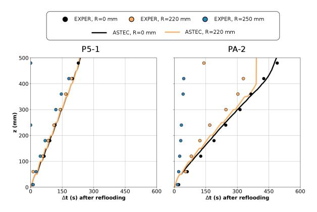
Figure 4: Predicted vs. Experimental quench front evolution for the tests P5-1 and PA-2.
