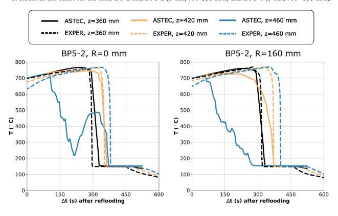
Figure 9: Evolution of computational and experimental debris temperatures at selected radial and axial locations for the test BP5-3.
