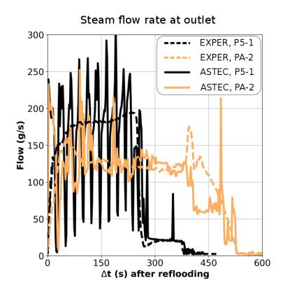
Figure 5: Predicted vs. Experimental evolution of the steam flow rate at the outlet for tests P5-1 and PA-2.
