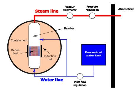
Figure 1: Schematic view of the PEARL facility.
