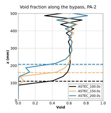
Figure 16: Predicted void fraction profiles along the bypass as a function of time for the test PA-2. Horizontal dashed lines represent the location of the quench front in the outermost bed channel at the times when the void fraction profiles are plotted.
