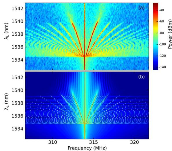
**Figure 1.** Radio-frequency spectrum of the resonator's output light, showing the formation of a comb around its mechanical eigenfrequency as function of the input laser wavelength. (a) Experiment. (b) Model.
