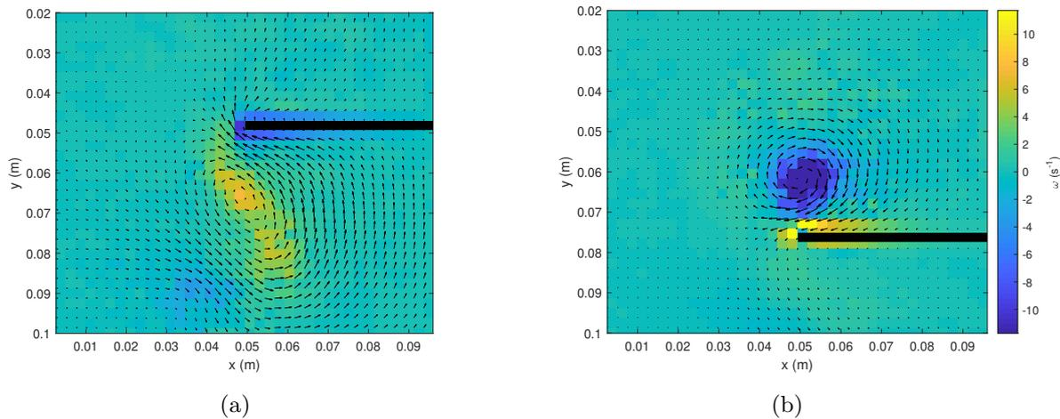
**Figure 1.** Velocity fields (arrows) and vorticity fields  $\omega$  (color scale) for  $A = 1.4$  cm,  $D = 10$  cm,  $f = 0.3$  Hz and  $e = 0.2$  cm. The fields are obtained by phase-averaging PIV results over 20 oscillations. The vortex rings created at the bottom of the disc (a) and the top (b) are asymmetric. We only show half of the disc as the flow is considered axisymmetric around the axis of the disc.
