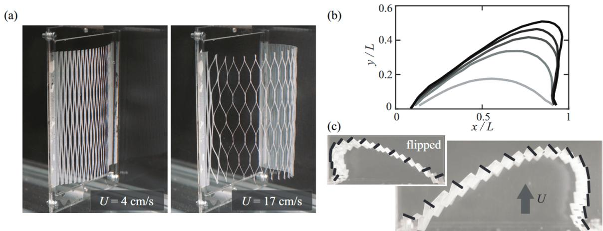
**Figure 1.** (a) Deployment in a water crossflow. (b) Typical shape profiles extracted from top-view pictures of the structure of length  $L$ , when increasing the flow speed  $U = [4, 8, 13, 17, 21] \text{ cm/s}$  (denoted by the grayscale). (c) The tilting of buckled cut units (outlined in black) induces tangential fluid forces, resulting in asymmetric profiles prescribed by the buckling direction (reversed in the inset)
