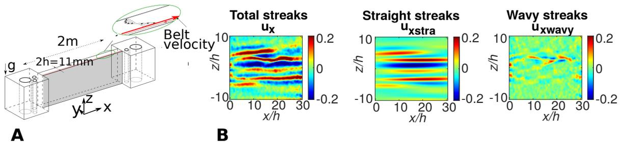
**Figure 1.** A: sketch of the experiment. B: streamwise fluctuation velocity  $u_x$ , made dimensionless using the belt velocity, at  $Re=500$  and spatial filtering separating the straight and wavy components of the streaks.
