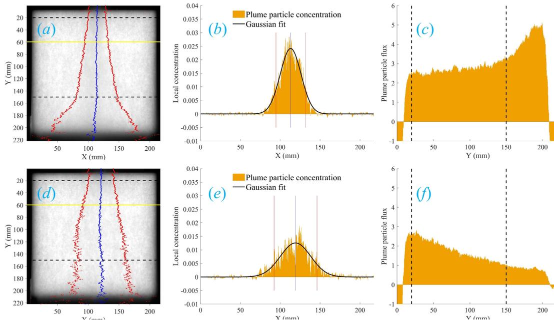
**Figure 1.** Plume particle concentration measurement, working zone between dash lines. First row, plastic beads, second row, salt, (a) and (d) Plume particle middle line and half width, (b) and (e) Plume particle profile fit for the yellow line, the red and blue line represent what shows in (a) and (d), (c) and (f) Plume particle flux change along vertical direction.
