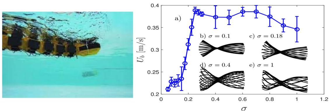
**Figure 1.** Left: the robot *Agnathax* [1] with its lateral force sensors. Right: transition of the robot's velocity  $U_b$  as a function of the weight of the sensory feedback in the oscillator chain. The body shapes are represented in black, indicating the transition from oscillating to undulating swimming modes.
