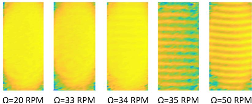
**Figure 1.** Color map of the velocity gradient measured by DWS on the surface of the Taylor–Couette cell. For each map, blue corresponds to the lowest values of the velocity gradient while red corresponds to the highest values. In our setup, the threshold is at  $\Omega = 34$  RPM, where we can start to distinguish the Taylor vortices.
