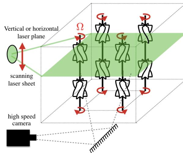
**Figure 1.** Sketch of the experimental set up. A tank of  $15 \times 15 \times 15$  cm is forced with 8 chiral helices, setting an integral length scale  $l_0 \approx 6$  mm significantly smaller than the system size.
