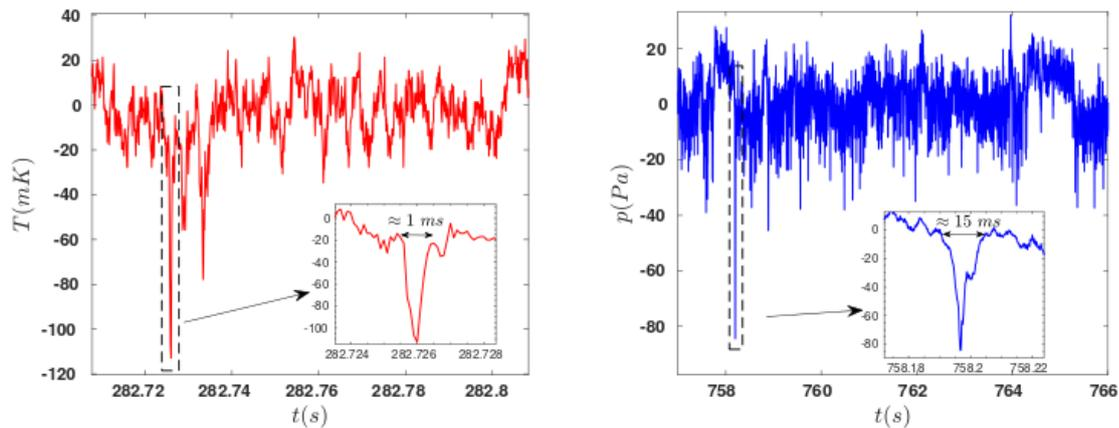
**Figure 1.** (a) Time series of temperature fluctuations measured in the bulk. (b) Time series of pressure fluctuations measured at the boundary. Inset figures show the zoom of one negative peak observed in temperature and pressure fluctuations.
