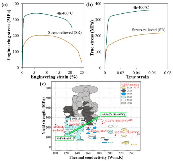
Figure 1: Typical (a) engineering and (b) true tensile stress-strain curves of LPBF Al-Fe-Zr in the stress-relieved (SR) and peak-aged conditions. (c) Ashby chart of yield strength as a function of thermal conductivity plotted with CES Selector GRANTA 2010, showing typical performance of wrought Al alloy series and the novel Al-Fe-Zr introduced in this work.
