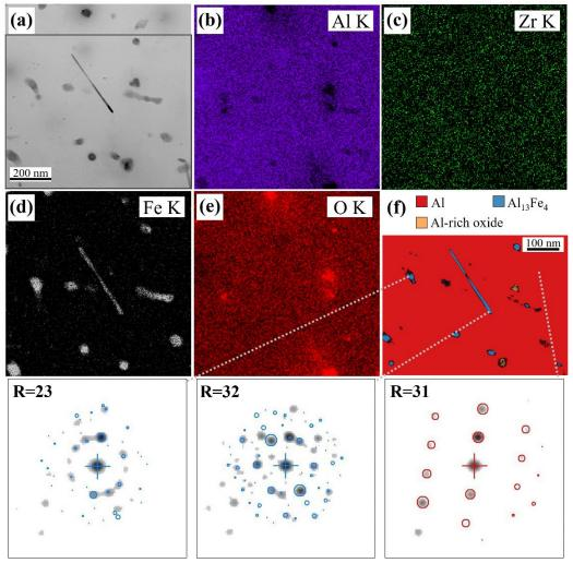
Figure 4: Local solute enrichments and phase distribution of a region of interest in the CZ after ageing at 400°C for 4h. (a) Virtual Bright Field image. EDS maps of the following elements: (b) Aluminium, (c) Zirconium, (d) Iron and (e) Oxygen. (f) Phase map showing the morphology and distribution of phases present within the frame highlighted in (a). The phase reliability in grey scale is overlaid on the map. Selected nanodiffraction patterns are displayed with their corresponding R index.
