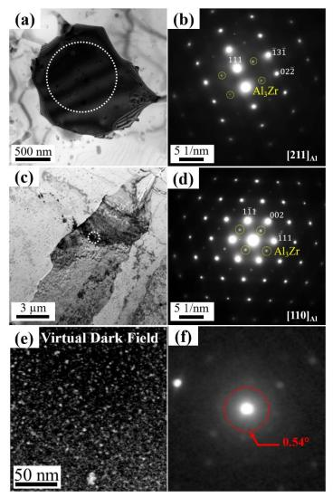
Figure 5: TEM imaging in zone axis of the aged sample: (a, b) bright field image within the FEZ and its associated SAED pattern, (c, d) corresponding image and pattern for the CZ.(e) Virtual Dark Field image within the CZ generated with ACOM and the virtual aperture displayed in (f) on an individual nanodiffraction pattern.
