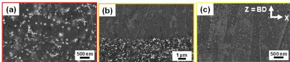
Figure 2. SEM-BSE micrographs taken in different regions of interest: (a) in the EZ ; (b) in the TZ ; (c) in the CZ.
