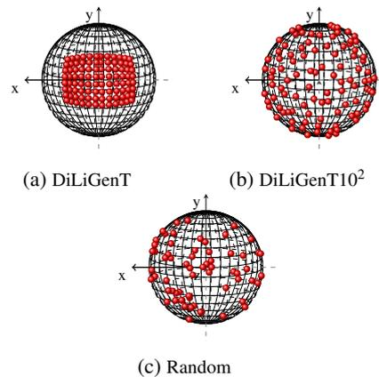
Figure 3: Distribution of illumination directions in the real *DiLiGenT* and *DiLiGenT10<sup>2</sup>* datasets, and an example of a random distribution. The  $z$ -axis corresponds to the optical axis of the camera, with the imaged object at coordinates  $(0, 0, 0)$ .
