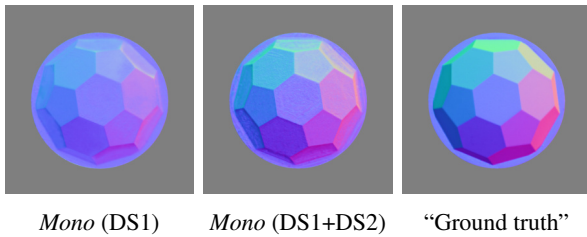
Figure 9: Results of our mono-scale architecture on the copper hexagon from [31]. Since the new dataset (DS2) contains much more metallic objects than the existing one (DS1), training on our new dataset yields largely improved results.
