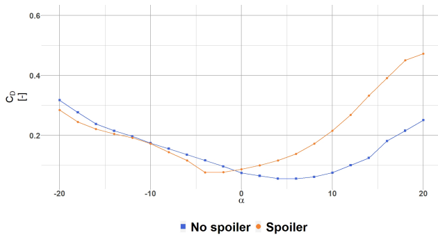
Figure 8. Drag coefficient polar for the radial position R6 ( \frac{r}{R} = 13\% ). The blue square (blue ■) shows the C_D for the no spoiler case, and the orange dot (orange ●) shows the C_D for the spoiler case.
