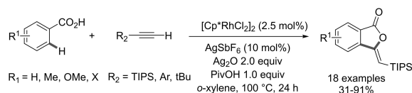
Scheme 31. Preparation of 3-ylideneephthalides via a Rh-catalyzed oxidative coupling of benzoic acids with terminal alkynes.
