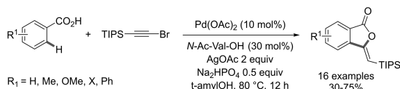
Scheme 35. Preparation of 3-ylidenephthalides via a Pd(II)-catalyzed ortho -alkynylation – annulation reaction of aromatic acids with bromoalkynes.
