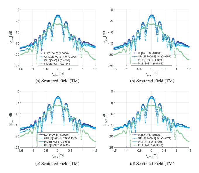
**Figure 4.** Modulus of the scattered field in decibel scale  $(10 \log_{10} |\psi_{\text{sca}}|)$  versus the observation abscissa  $x_{\text{obs}} \in [-L/2; L/2]$  and for an observation height  $z_{\text{obs}} = 470 \text{ mm}$ . The frequency is f = 2 GHz and the orders P and Q vary. (a) P = 1 and Q = 0. (b) P = Q = 1. (c) P = 2 and Q = 0. (d) P = 2 and Q = 1.
