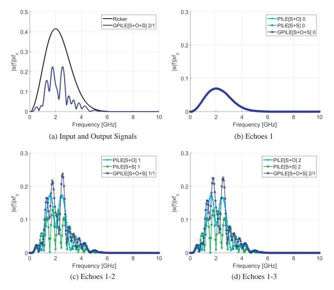
Figure 7. Frequency responses of the modulus of the scattered field.  $x_{obs} = 0$ ,  $z_{obs} = 470$  mm. (a) Input and Output signals. (b) First echo (P = 0). (c) First two echoes (P = 1). (d) First three echoes (P = 2).
