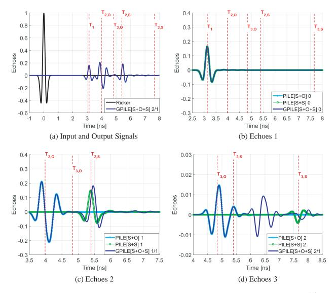
**Figure 8.** Time responses of the modulus of the scattered field.  $x_{obs} = 0$ ,  $z_{obs} = 470$  mm. (a) Input and Output signals. (b) First echoes (P = 0). (c) Second echoes (P = 1). (d) Third echoes (P = 2).
