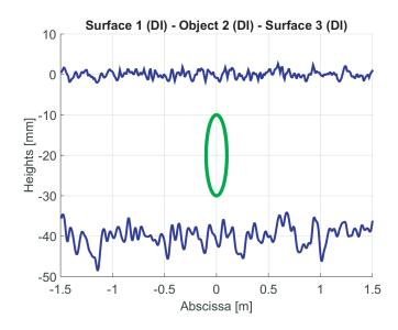
Figure 2. Surface heights versus their abscissa for Gaussian PDF and ACF, with  $\sigma_{h,1} = 1 \text{ mm}$  and  $\sigma_{h,3} = 2.5 \text{ mm}$ ,  $L_{ch,1} = 15 \text{ mm}$  and  $L_{ch,3} = 30 \text{ mm}$ . The center of the cylinder is C = (0, -0.5H), and a = 100 mm and b = 10 mm.
