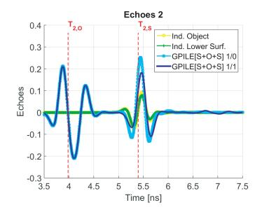
Figure 9. Time response of the modulus of the scattered field: Direct and Indirect contributions.  $x_{obs} = 0$  and  $z_{obs} = 470$  mm.
