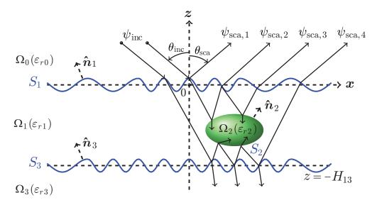
Figure 1. Electromagnetic scattering from an object buried between two 1-D rough surfaces (2-D problem: plane  $(\hat{\mathbf{x}}, \hat{\mathbf{z}})$ ).
