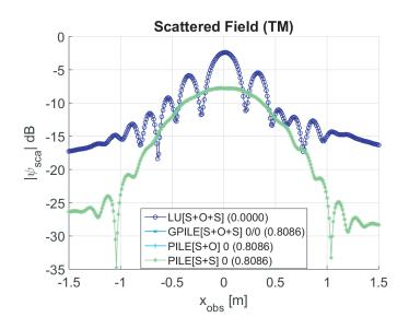
Figure 3. Modulus of the scattered field in decibel scale  $(10 \log_{10} |\psi_{\rm sca}|)$  versus the observation abscissa  $x_{\rm obs} \in [-L/2; L/2]$ , for an observation height  $z_{\rm obs} = 470$  mm. The frequency is f = 2 GHz and P = 0.
