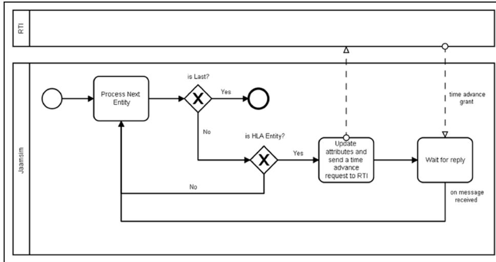
**Figure 6.** BPMN process of JaamSim developed HLA module.
