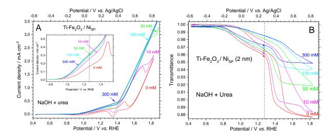
(A) Voltammetry under illumination of FTO/Ti-Fe<sub>2</sub>O<sub>3</sub>/Ni<sub>PEC</sub> (8.75 mC cm<sup>-2</sup>) in NaOH and different urea concentrations; (B) Transmittance measured *in situ* during voltammetry. [NaOH] = 1 mol L<sup>-1</sup>; [urea] = 0, 10, 50, 150 and 300 mmol L<sup>-1</sup>. Scan rate: 2 mV s<sup>-1</sup>. Illumination: AM1.5G, 1000 W m<sup>-2</sup>.
