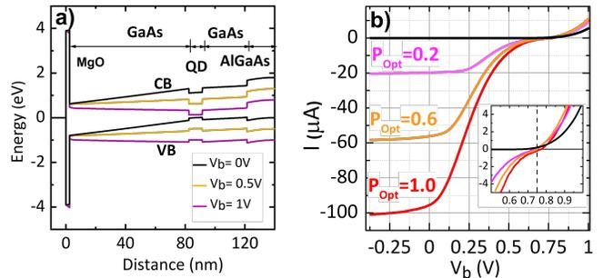
FIG. 1. a) Band profile of the semiconductor stack for different electrical bias ( $V_b$ ) applied to the substrate, the ferromagnetic metal top layer being grounded; b)  $I(V)$  curves in the dark (black) and under light excitation with powers in the ratio 1.0/0.6/0.2; inset: zoom on the high-impedance forward domain around  $V_b = 0.75 \text{ V}$ .
