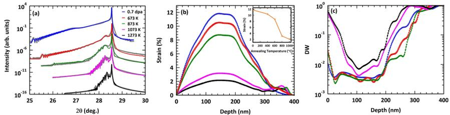
**Fig. 3** (a) HR-XRD profiles of 4H-SiC irradiated with fluence of  $6.7 \times 10^{14}$  ions/cm<sup>2</sup> (0.7 dpa) using 300 keV Ar ions and annealed at various indicated temperatures. Colored lines are results of simulations and the grey lines represent the experimental data. (b) and (c) are the corresponding Strain and DW depth profiles. Inset to (b) shows the variation of strain(%) at 175nm with annealing temperatures. Connecting line is drawn to guide the eyes.
