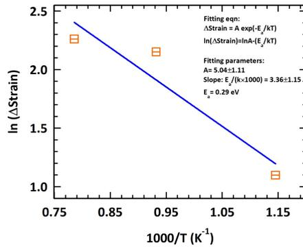
**Fig. 4** Arrhenius plot of strain recovery for thermally annealed 0.7 dpa 4H-SiC. The change in strain(%) w.r.t pristine is calculated at 175nm using Figure 3(b). The blue connecting line is the line of best fit.
