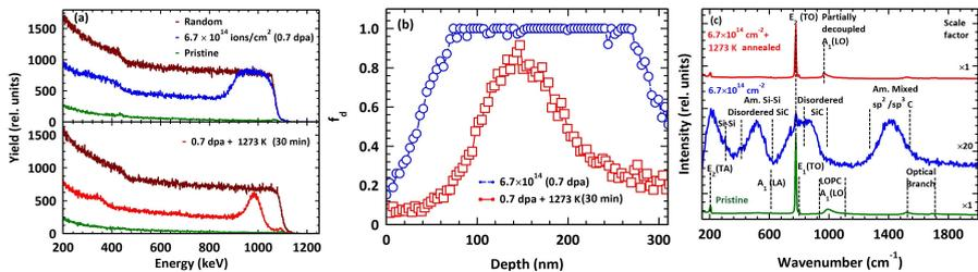
**Fig. 1** (a) RBS/C spectra recorded on 4H-SiC after 300 keV Ar irradiation with fluence of  $6.7 \times 10^{14}$  ions/cm<sup>2</sup>, and after subsequent thermal annealing of the sample at 1273 K for 30 mins and (b) is the corresponding depth profiles of disorder ( $f_d$ ) extracted using DICADA. [20] (c) Raman spectra of the pristine, irradiated and annealed sample.
