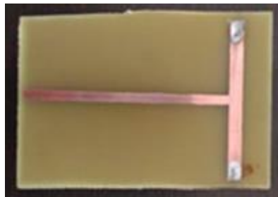
Fig. 2. T- resonator built in FR4 material.
