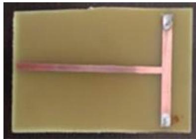
Fig. 2. T- resonator built in FR4 material.
