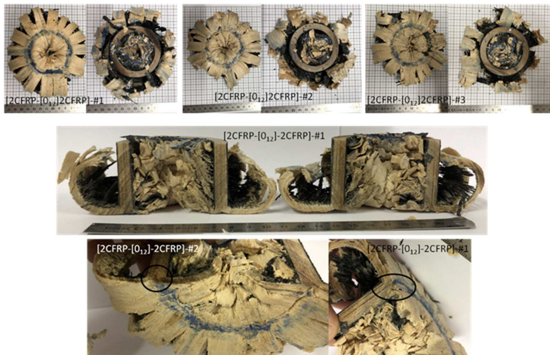
Figure 5. Post-mortem failure analysis of birch and carbon fiber sandwich tubes (a) overview (b) half-tubes.
