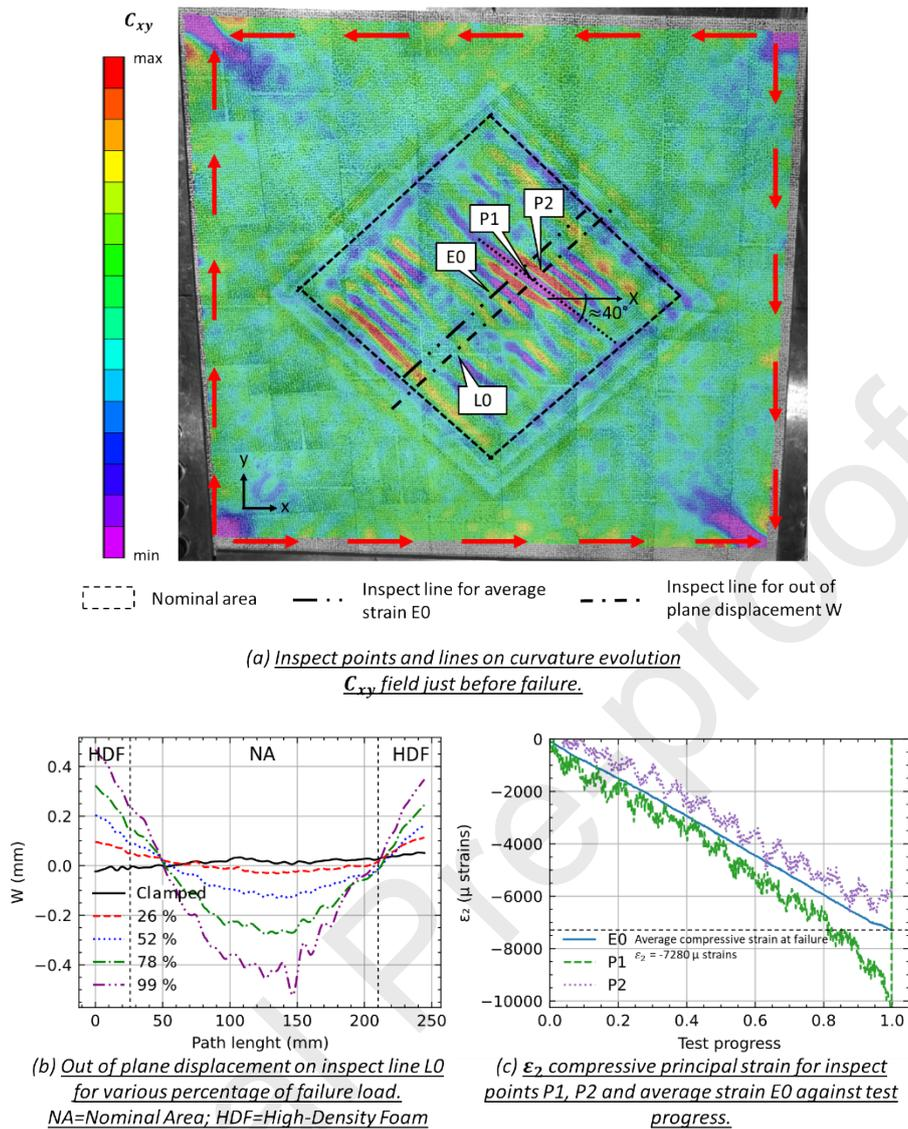
Figure 24: Specimen N29\_D3 local behaviour.
