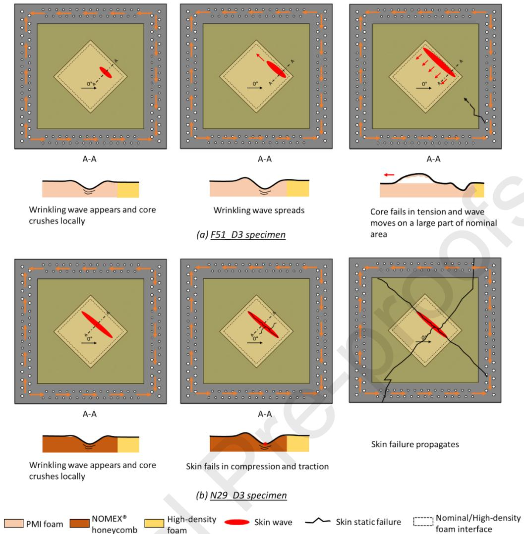
Figure 25: Failure scenario for specimen under shear.
