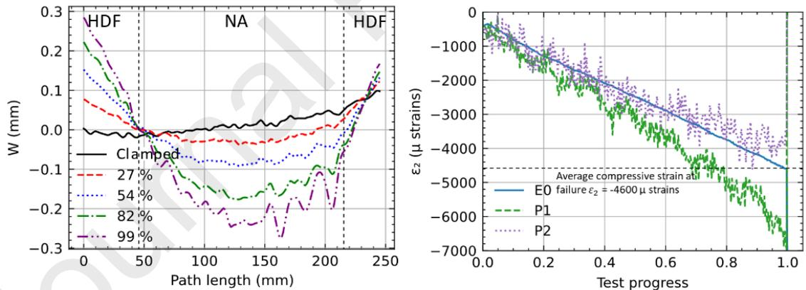
(b) Out of plane displacement on inspect line LO for various percentages of failure load.
