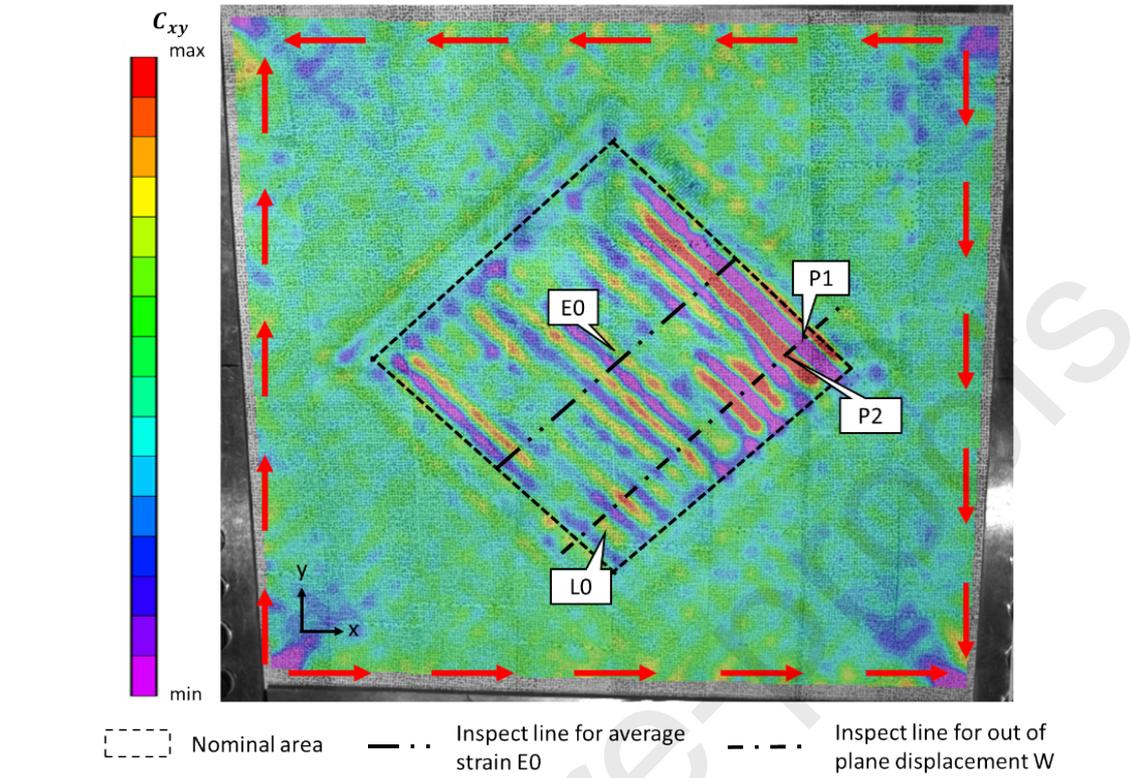
(a) Inspect points and lines on curvature evolution  $C_{xy}$  field just before failure.
