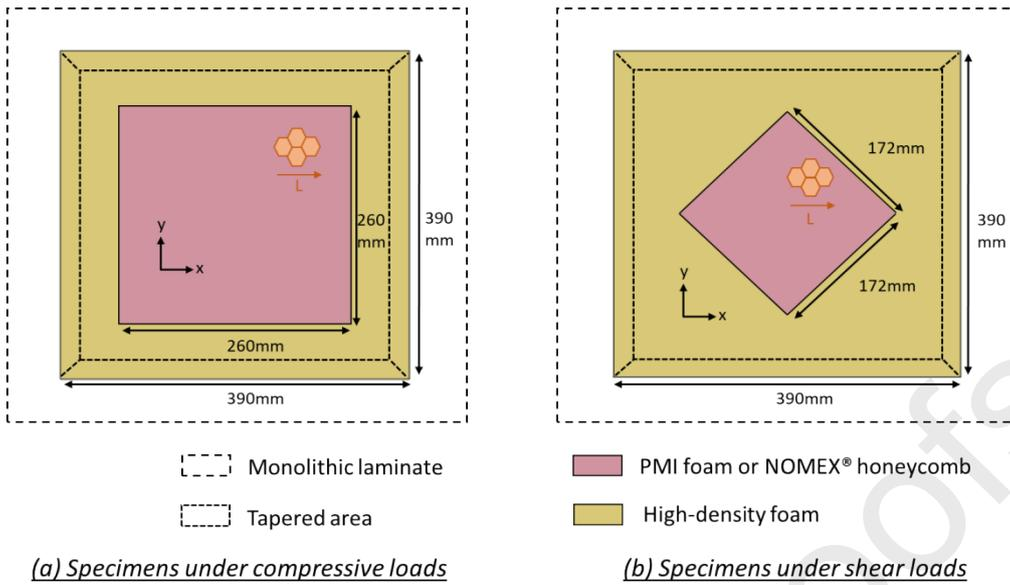
Figure 7: Definition of the cores of the specimens.
