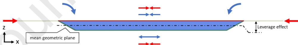
Figure 5: Bending effect on asymmetric sandwich structure.
