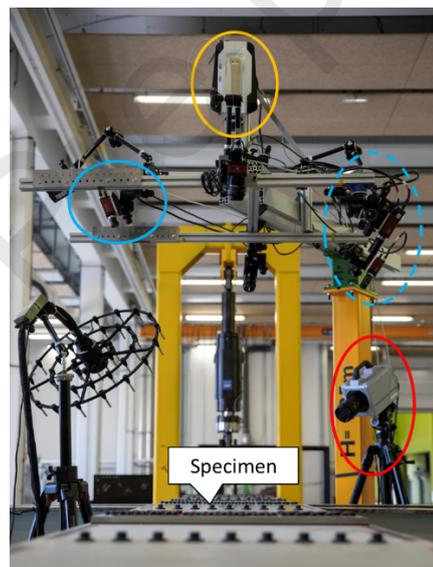
Figure 9: Camera set up on the VERTEX test bench.
