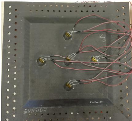
(a) "Rosette" gauges in lower skin of specimens tested under compression
