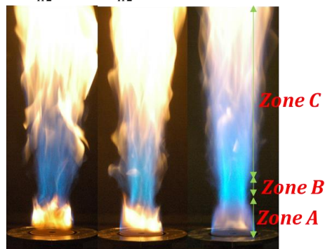
Figure 1. a. Configuration of canonical non-premixed bluff-body burner used in this study ( D_a = 55 \text{ mm} ; D_b = 48 \text{ mm} ; t_b = 20 \text{ mm} ); b – Time averaged flow field with distinct flow regions; c – Direct photographs of flames across various H 2 addition levels.
