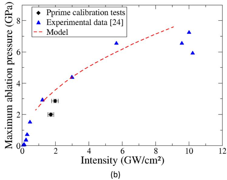
Fig. 7: Maximum ablation pressure measurements as a function of intensity for water confinement and comparison with the analytical model (with  $\alpha = 0.2$ ) (a) ; for glass confinement and comparison with the analytical model (with  $\alpha = 0.15$ ) (b).
