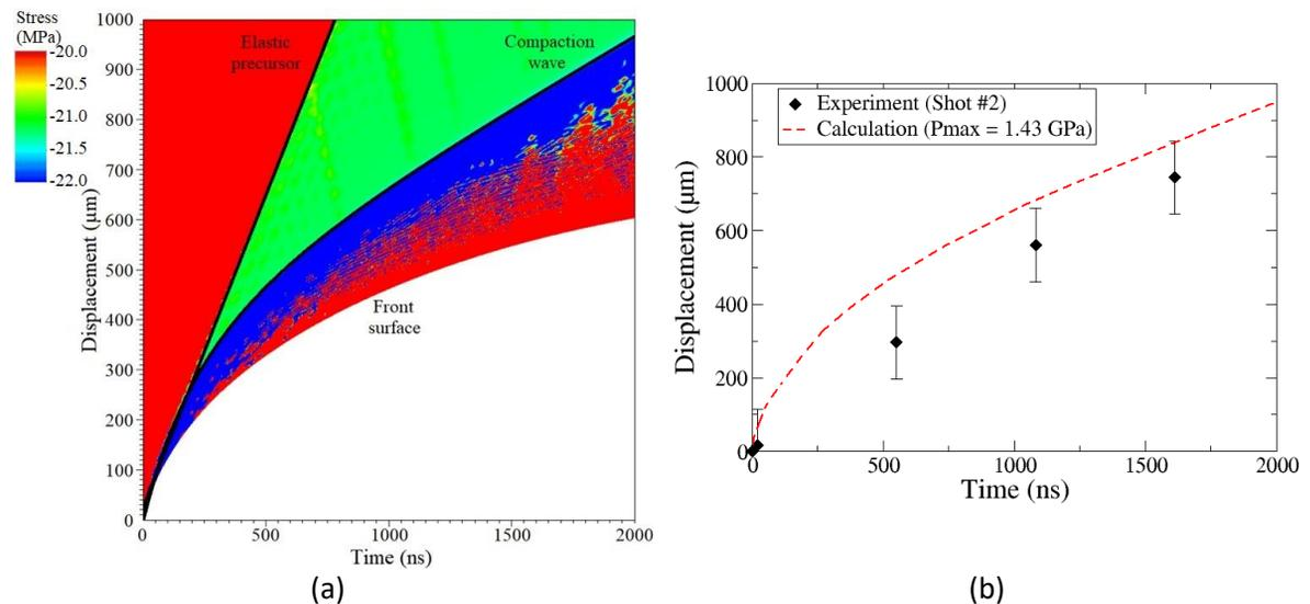
Fig. 15: Simulation of the ESRF experiment #2. (a): distance-time diagram showing wave propagation, with pressure contours bounded between 20 MPa (red) and 22 MPa (blue), and (b): computed
