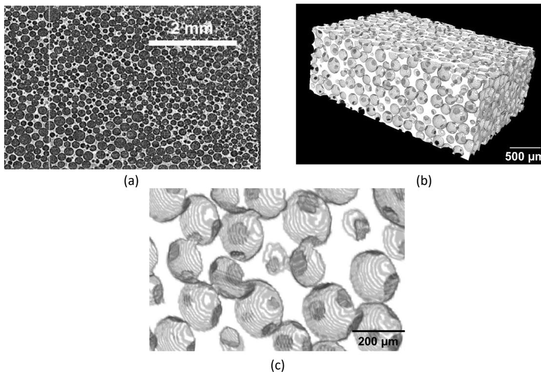
Fig. 1: Initial mesostructure of the polyurethane foam: 2D section extracted from X-ray tomography (a), 3D X-ray tomography (b), and closer view (c) showing the presence of small holes interconnecting pores to each other.
