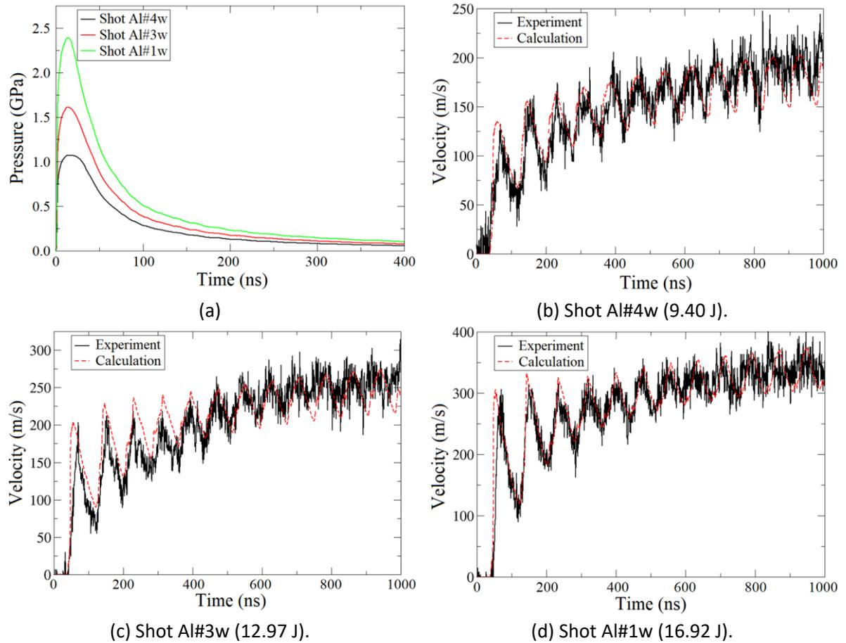
Fig. 6: Loading pressure profiles for three typical laser shots (a) obtained from comparisons between calculated and measured velocity profiles at the free surface of aluminum samples (b-d).
