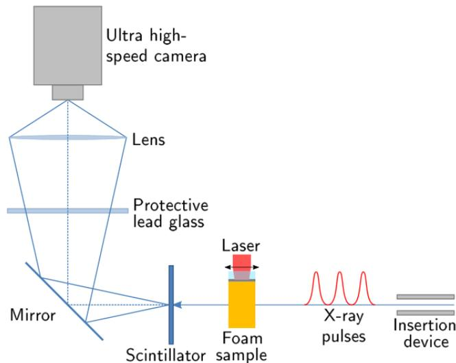
Fig. 2: Experimental set-up for laser-driven shock experiments performed at the ESRF. After crossing the foam sample, X-ray pulses are detected using a LYSO:Ce scintillator and a HPV-X2 Shimadzu ultra high-speed camera.
