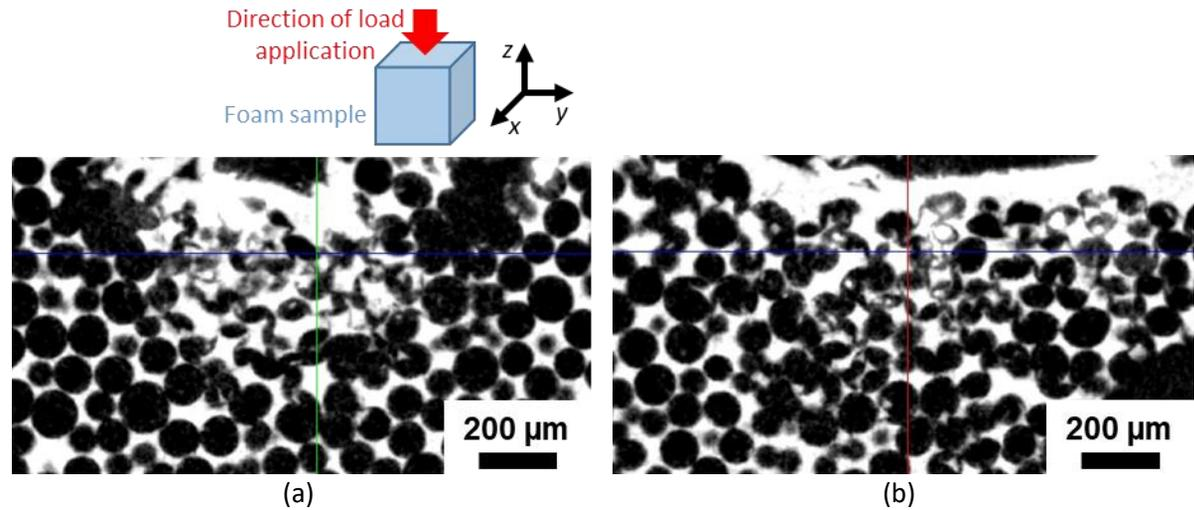
Fig. 11: Two sections in  $yz$  (a) and  $xz$  (b) orthogonal planes extracted from post-shock X-ray tomography of the foam sample recovered after the laser shot #3 at the ESRF, in water-confined geometry ( $E = 3.8$  J,  $D = 3$  mm).
