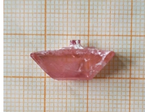
Fig. 1. A photograph of the as-grown 1.01 at.% Er 3+ :MgWO 4 crystal, the growth direction is along the [010] axis.
