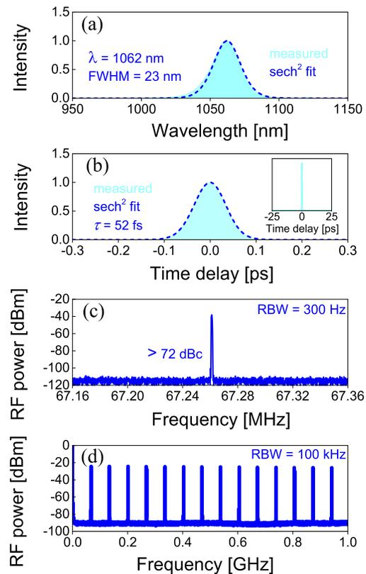
**Fig. 4.** ML Yb:GdCB laser with  $T_{OC} = 2.5\%$ . (a) Optical spectrum and (b) SHG-based intensity autocorrelation trace. *Inset*: autocorrelation trace on a time span of 50 ps. RF spectra: (c) first beat note at  $\sim 67.2$  MHz recorded with an RBW of 300 Hz, and (d) harmonics on a 1-GHz frequency span, RBW = 100 kHz.
