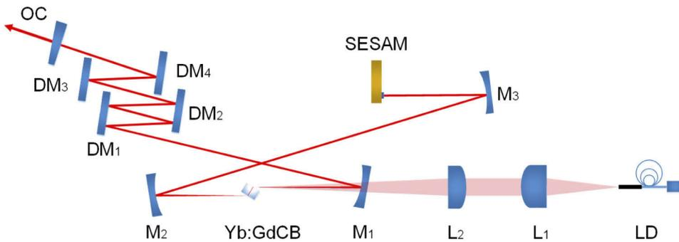
**Fig. 2.** Experimental setup of the ML Yb:GdCB laser. LD: fiber-coupled laser diode;  $L_1$ : aspherical lens;  $L_2$ : achromatic doublet lens;  $M_1 - M_3$ : concave mirrors;  $DM_1 - DM_4$ : flat dispersive mirrors; OC: output coupler; SESAM: SEmiconductor Saturable Absorber Mirror.
