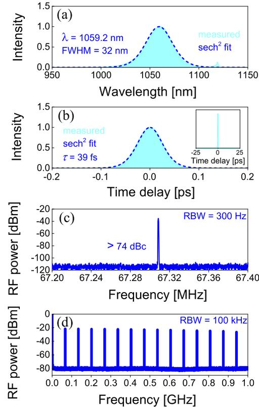
**Fig. 5.** ML Yb:GdCB laser with  $T_{OC} = 1.6\%$ . (a) Optical spectrum and (b) SHG-based intensity autocorrelation trace with a  $\text{sech}^2$ -fit. *Inset*: simultaneously measured long-scale autocorrelation trace for the time span of 50 ps. RF spectra of the Yb:GdCB laser: (c) first beat note at  $\sim 67.3$  MHz recorded with a RBW of 300 Hz, and (d) harmonics on a 1-GHz frequency span, measured with a RBW of 100 kHz.
