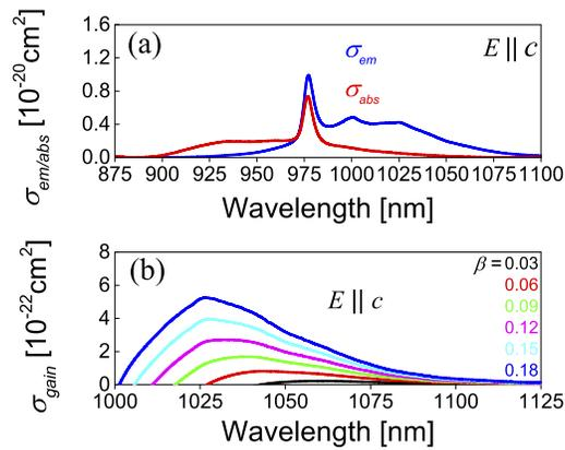
**Fig. 1.** Room-temperature spectroscopy of the Yb:GdCB crystal for light polarization  $E \parallel c$ : (a) absorption ( $\sigma_{\text{abs}}$ ) and stimulated-emission (SE,  $\sigma_{\text{SE}}$ ) cross-sections; (b) gain cross-sections ( $\sigma_{\text{gain}}$ ),  $\beta$  is the inversion ratio.
