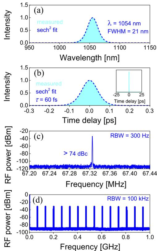
**Fig. 3.** ML Yb:GdCB laser with  $T_{OC} = 4\%$ . (a) Optical spectrum and (b) SHG-based intensity autocorrelation trace. *Inset*: autocorrelation trace on a time span of 50 ps. RF spectra: (c) first beat note at  $\sim 67.3$  MHz recorded with a resolution bandwidth (RBW) of 300 Hz, and (d) harmonics on a 1-GHz frequency span, RBW = 100 kHz.
