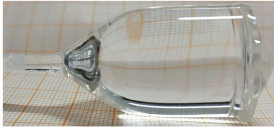
**Fig. 1.** Photograph of an as-grown 5 at.% Yb:GdCB crystal.
