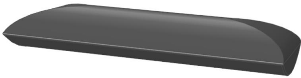
FIG. 4. Optimized pole design obtained from the original shape and additional geometric constraints leading to smoothing the profile and minimizing some harmonics. The shape is the result of an experimentation plan which takes 1 hour on a standard laptop (64 bits, 2.8 GHz, 32 Go RAM).
