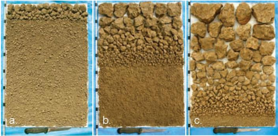
Figure 1: Visual key for scoring soil structure after a drop-shatter test. (a) Good, (b) moderate, and (c) poor physical condition. Reprinted from Shepherd et al. (2008).
