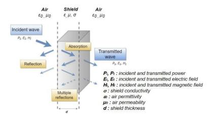
Figure 1: Schematic representation of different mechanisms for electromagnetic shielding.
