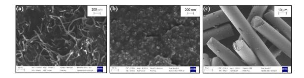
**Figure 4:** SEM images of the fillers used for preparing our PMMA based composite materials: (a) MWCNT; (b) CB; (c) AgGF.
