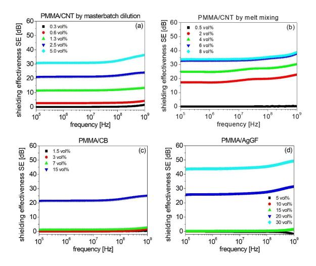
**Figure 5:** shielding effectiveness of (a) PMMA/CNT composite materials prepared by masterbatch dilution; (b) PMMA/CNT composite materials prepared by direct mixing; (c) PMMA/CB composite materials; (d) PMMA/AgGF composite materials, in dependence on frequency and at different filler concentrations, as indicated.
