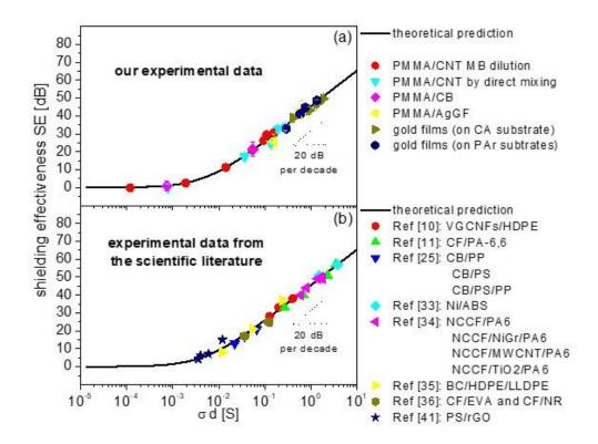
**Figure 6:** Shielding effectiveness as a function of the product between conductivity  $\sigma$  and sample thickness d for: (a) our own experimental data at 100 kHz (b) data from the scientific literature, as indicated. The continuous black lines correspond to the theoretical curve predicted by eq. 4.
