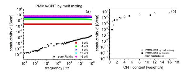
**Figure 3:** (a) conductivity spectra of PMMA/CNT composite materials prepared by melt mixing; (b) percolation curves (conductivity  $\sigma$ ' as a function of filler concentration) for PMMA/CNT composite materials prepared by direct melt mixing and by masterbatch dilution. The star symbols correspond to the data reported in ref. 42.
