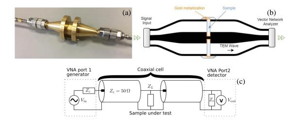
**Figure 2:** (a) the coaxial cell used in our study; (b) schematic representation of the coaxial measurement cell. (b) equivalent electric circuit representing a coaxial cell.
