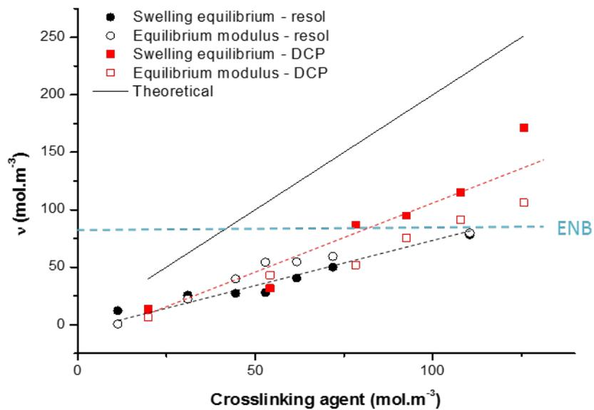
**Fig 2:** Variation of the density of elastically active chains ( $\nu_R$  and  $\nu_S$ ) versus the molar concentration of crosslinking agents. The density has been measured from equilibrium shear modulus (open symbols) and swelling equilibrium (full symbols).
