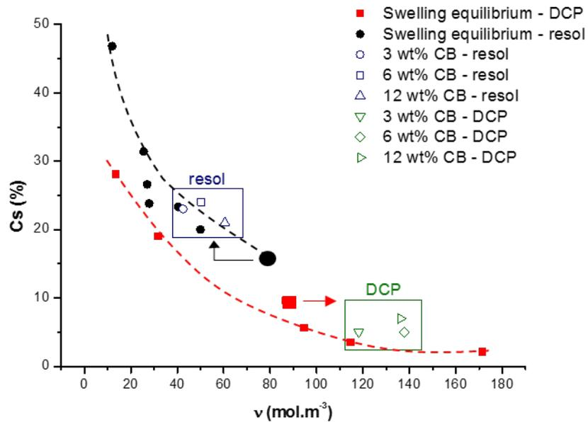
**Fig 6:** Influence of the carbon black filler (N550) on the compression set for the two types of crosslinking agents (resol and DCP). The trend curves are as shown in **Fig 3**. In the frame are the points obtained in the presence of CB filler.
