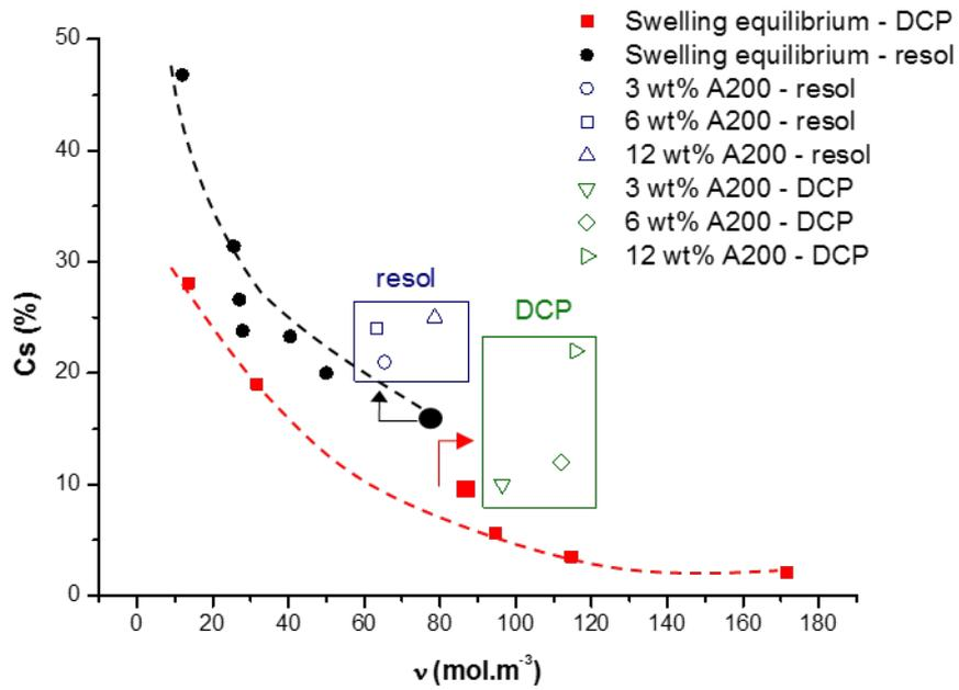
**Fig 7:** Influence of hydrophilic silica fillers Aerosil A200 on the compression set for the two types of crosslinking agents (resol and DCP). The trend curves are as shown in Fig 3. In the frame are the points obtained in the presence of these silica fillers.
