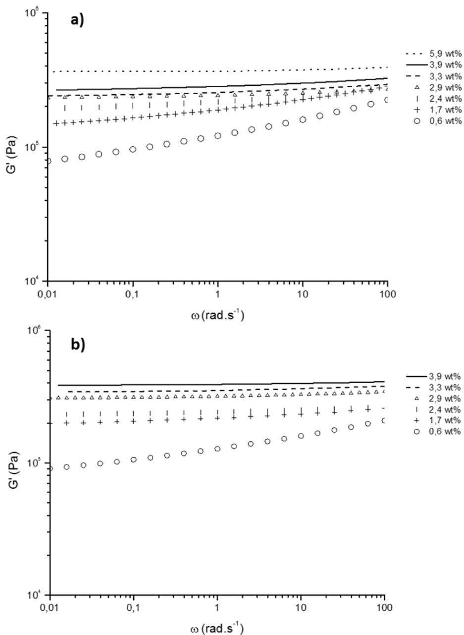
**Fig S 1:** Variation of the storage shear modulus versus frequency for crosslinked EPDM samples: **a)** EPDM crosslinked with resol, **b)** EPDM crosslinked with dicumyl peroxide.
