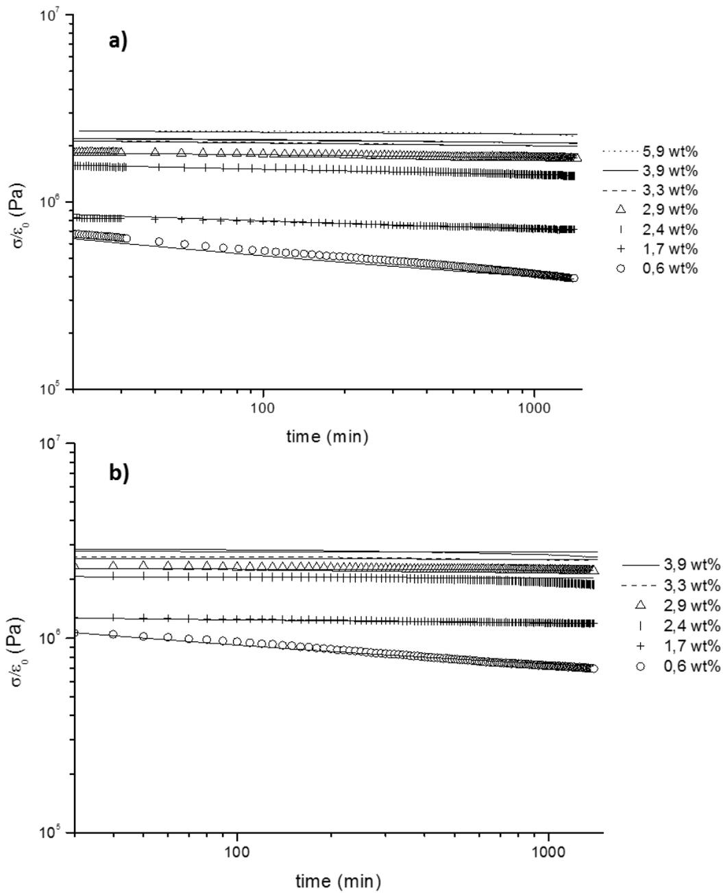
**Fig S 2:** Stress relaxation at the long time ( $\Delta t = 24$ hours,  $T = 100^\circ\text{C}$ ,  $\varepsilon_{0,n} = 0.25$ ), **a)** EPDM crosslinked with resol, **b)** EPDM crosslinked with dicumyl peroxide. The curves show the modelling from the Chasset-Thirion equation.
