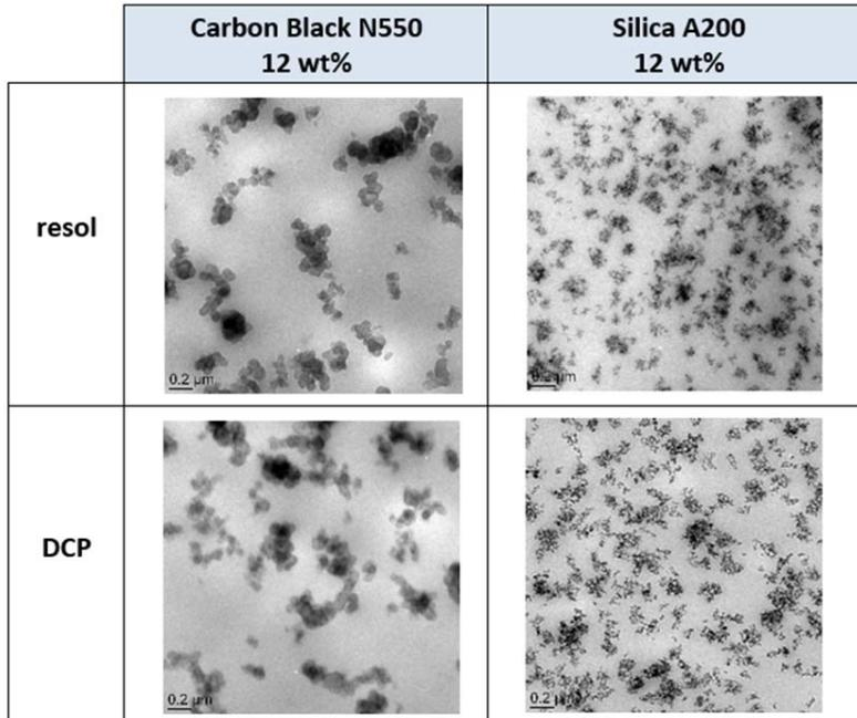
**Fig 8:** TEM images of carbon black and silica fillers dispersed in crosslinked EPDM samples. The crosslinking densities of these samples measured by swelling equilibrium are the following: resol/CB:  $60 \text{ mol.m}^{-3}$ ; resol/silica:  $79 \text{ mol.m}^{-3}$ ; DCP/CB:  $136 \text{ mol.m}^{-3}$ ; DCP/silica:  $116 \text{ mol.m}^{-3}$ .
