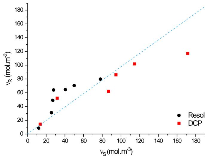
**Fig 1:** Plot of  $v_R$  versus  $v_S$ . Comparison between elastically active chains calculated from the equilibrium shear modulus and the swelling equilibrium.
