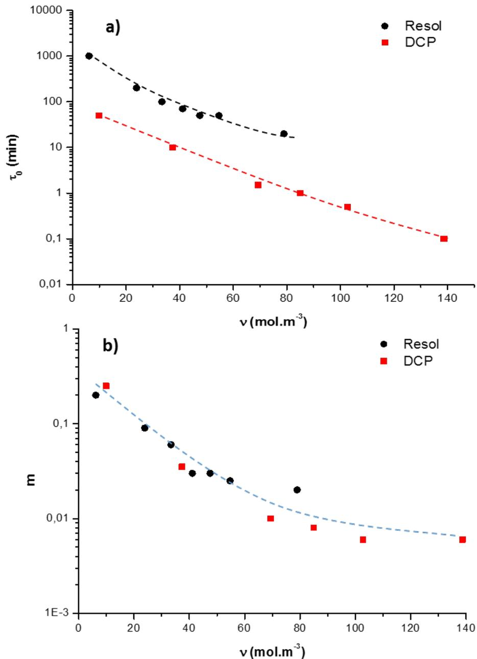
**Fig 5:** Variation of the exponents of the Chasset-Thirion equation. **a)** Variation of the relaxation time of the dangling end chains and **b)** Variation of  $m$  versus the density of elastically actives of EPDM crosslinked either by DCP or resol.
