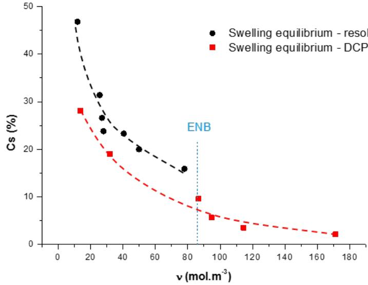
**Fig 3:** Variation of the compression set (Cs%) of crosslinked EPDM samples versus the density of the elastically active chains for the two types of crosslinking agents. The density has been measured from swelling equilibrium experiments
