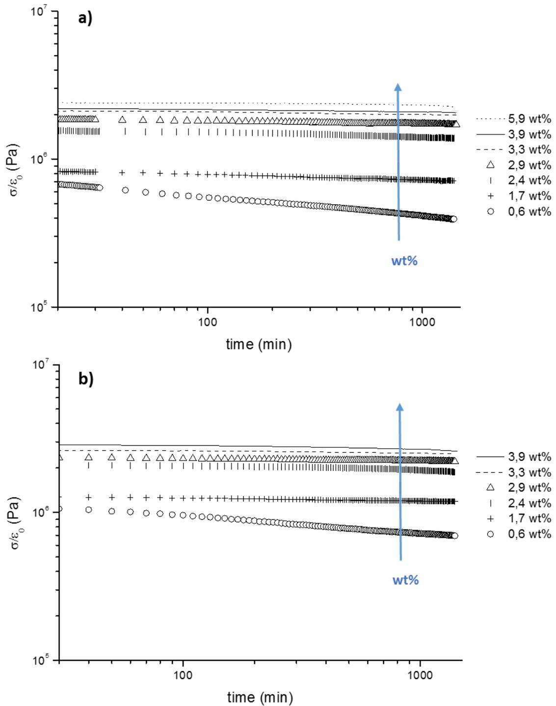
**Fig 4:** Variation of the stress relaxation versus the time. **a)** Networks crosslinked with the resol and **b)** crosslinked with the DCP
