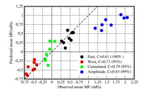
**Figure 4.** Scatter plot of the momentum fluxes measured by the balloon versus parametrized. Eight values are averages for the eight balloon flights. Significant test are for the correlation between the values, significance is estimated via a Pearson test with 6 degrees of freedom.
