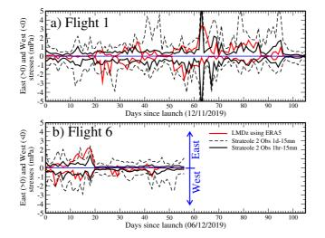
Figure 2. Comparison between daily averaged values of the eastward and westward MFs measured by the balloons and estimated by the GW scheme at the balloon location and altitude. Red curves are for the GW scheme predictions using ERA5, black curves are for the observed MFs due to the 15mn-1hr GWs, the thin dashed black curves are for MFs due to the 15mn-1day GWs.
