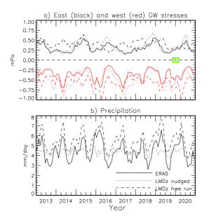
Figure 7. Time series of the z = 20km zonal mean zonal non-orographic GW stresses and of the zonal mean precipitation averaged over the equatorial band (5°S-5°S). Same input datas as in Figure 6.
