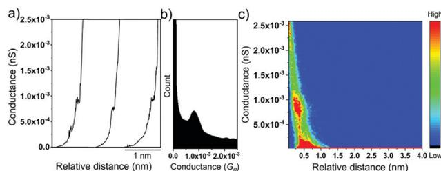
Fig. 1 (a) Typical  $I(s)$  curves of Au/OT6/graphene junctions collected by the  $I(s)$  method at 300 mV; (b) the one-dimensional (1D) histogram of single molecule conductance of OT6 constructed from about 500 curves; (c) the two-dimensional (2D) histograms of the conductance of OT6.
