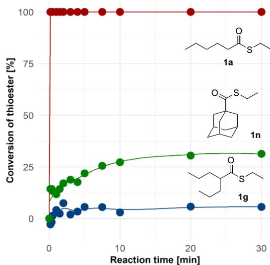
**Figure 1.** Conversion of different thioesters under catalytic conditions.
