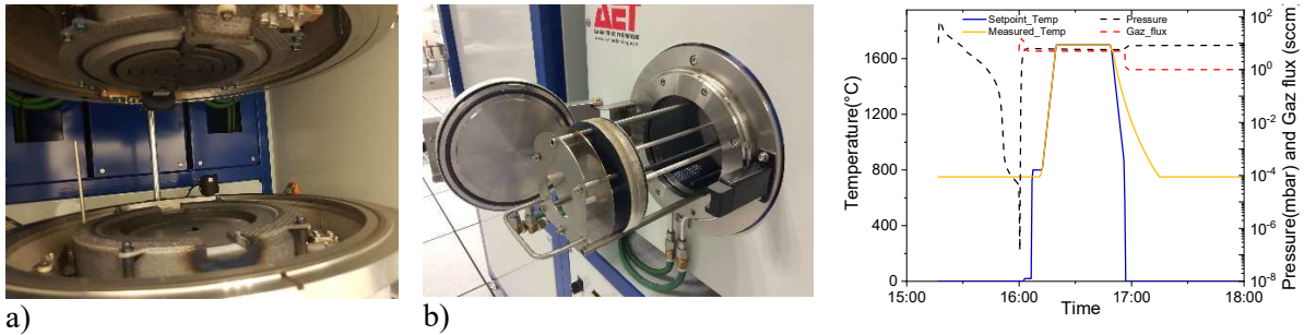
Fig. 1. 150 mm AET furnace for this study: RTP chamber with graphite resistors (a), pyrolyzed quartz chamber (b) and typical temperature and Ar pressure profiles for the RTP 1700°C 30 min plateau.
