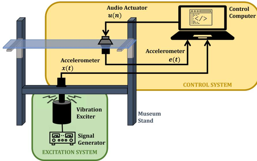
Figure 4: Schematic representation of the experimental bench.
