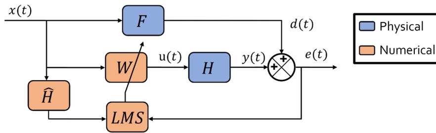
Figure 2: Block diagram of the FXLMS algorithm.  $x(t)$  represents the reference signal and  $e(t)$  is the error signal.  $F$  and  $H$  are respectively the primary and secondary path, while  $\hat{H}$  is the estimation of the secondary path.  $W$  is the control filter, updated at every new time sample following a Least Mean Square ( $LMS$ ) optimisation.
