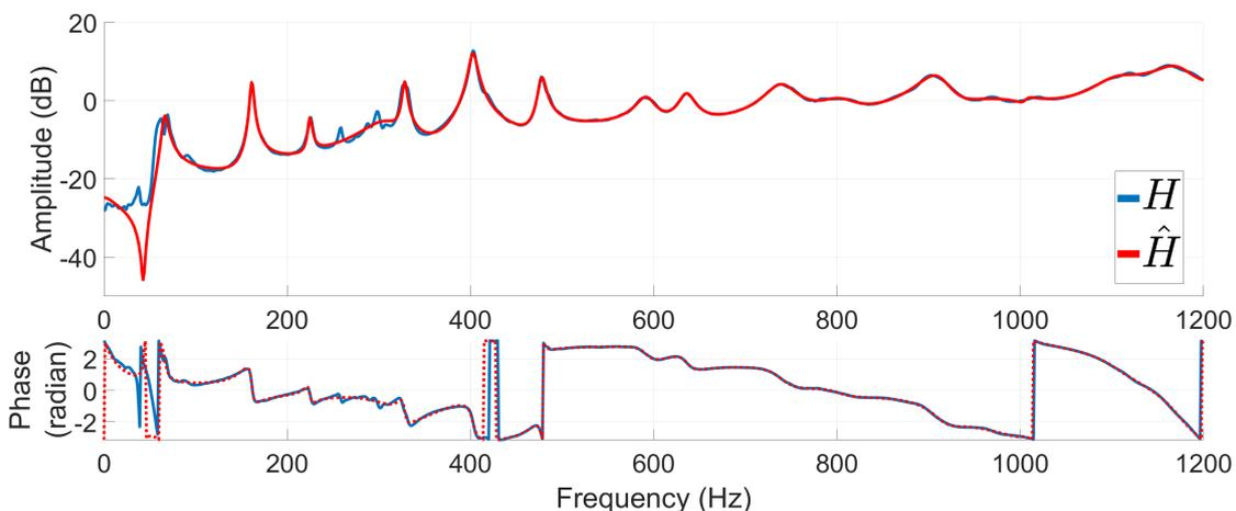
Figure 5: Frequency response of the secondary path  $H$  and of its identification ( $\hat{H}$ ).
