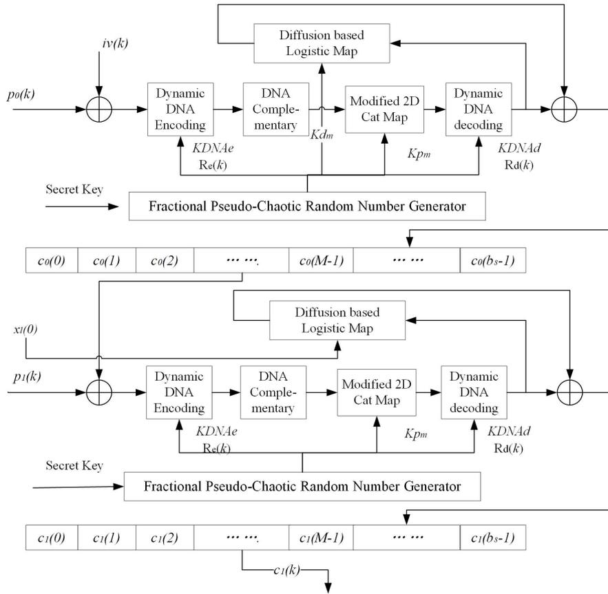
**Fig. 7** Encryption structure of the cryptosystem
