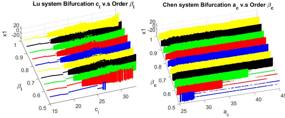
**Fig. 3** Bifurcation diagram of Lu and Chen systems of different fractional orders
