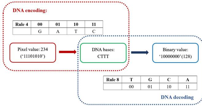
**Fig. 1** Example of DNA encoding and decoding
