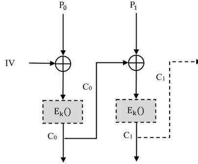
Fig. 6 CBC mode encryption structure
