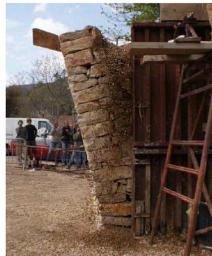
Fig. 5. Experimental toppling failure obtained by Colas [39].
