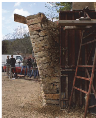
126 127 Figure 5: Experimental toppling failure obtained by Colas [39]
