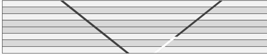
Figure 12: Scarf repair with bondline flaw
