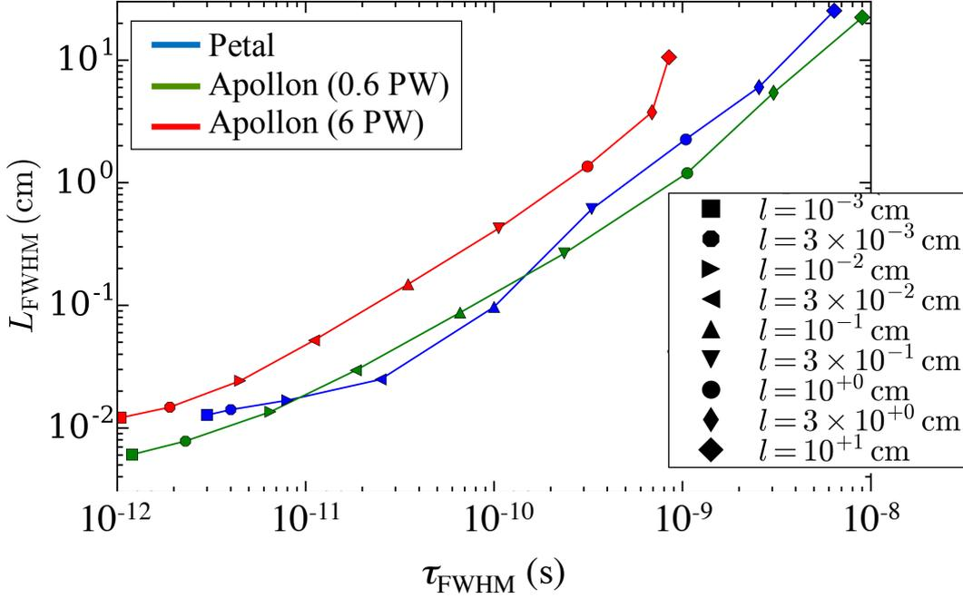
Figure 13: Transverse size vs duration of the simulated neutron beam in the LMJ-PETAL, 0.6 PW Apollon and 6 PW Apollon cases, and for various thicknesses, as indicated.
