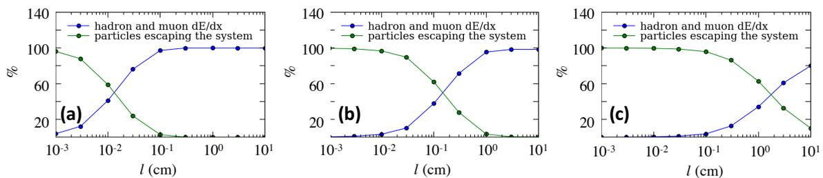
Figure 10: Energy fraction of the incident protons dissipated by nuclear reactions (blue) and transmitted through the target (green), as a function of the thickness  $l$  of the Pb converter target. Panels (a), (b) and (c) correspond, respectively, to the LMJ-PETAL, **0.6 PW Apollon** and **6 PW Apollon** lasers.
