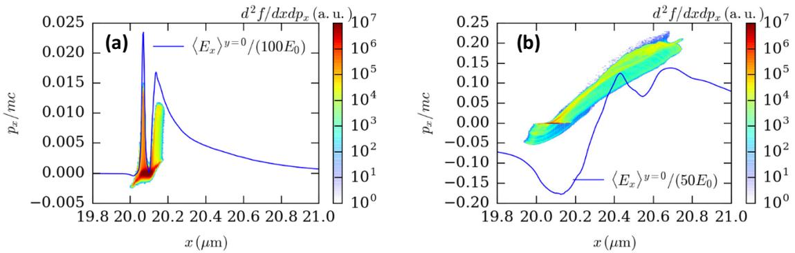
Figure 6: Proton acceleration using the 0.6 PW Apollon laser parameters:  $x - p_x$  proton phase spaces at (a)  $t = -20 \text{ fs}$  and (b)  $t = +4 \text{ fs}$  (here  $t = 0$  corresponds to the on-target laser pulse maximum). The blue line is the laser-cycle-averaged longitudinal electric field,  $\langle E_x \rangle$ , normalized to (a)  $100 E_0$  or (b)  $50 E_0$  for readability ( $E_0 = 3.2 \times 10^{12} \text{ Vm}^{-1}$ ).
