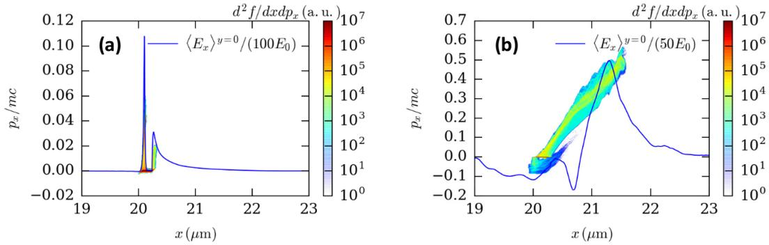
Figure 7: Proton acceleration using the 6 PW Apollon laser parameters:  $x - p_x$  proton phase spaces at (a)  $t = -20$  fs and (b)  $t = +4$  fs (here  $t = 0$  corresponds to the on-target laser pulse maximum). The blue line is the laser-cycle-averaged longitudinal electric field,  $\langle E_x \rangle$ , normalized to (a)  $100 E_0$  or (b)  $50E_0$  for readability ( $E_0 = 3.2 \times 10^{12} \text{ Vm}^{-1}$ ).
