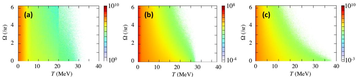
Figure 9: Energy-angle spectrum of the neutrons escaping from a **0.3 mm thick Pb converter target**. (a) The incident proton beam is that of the LMJ-PETAL PIC simulation. (b) Same with the **0.6 PW Apollon** laser parameters (c) Same with the **6 PW Apollon** laser parameters.
