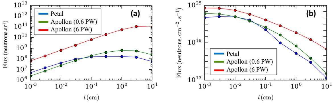
Figure 11: (a) Number (normalized to unit solid angle) and (b) maximum flux of the neutrons crossing the rear side of the Pb converter target, as a function of its thickness  $l$ . The incident proton beam is that predicted by PIC simulations in the LMJ-PETAL and 0.6-6 PW Apollon cases, as labeled.
