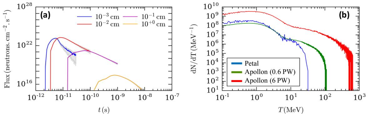
Figure 12: (a) Time-dependent neutron flux across the Pb converter backside for the LMJ-PETAL parameters. (b) Neutron energy spectra from a  $l = 0.3$  mm Pb target in the LMJ-PETAL and 0.6-6 PW Apollon cases.
