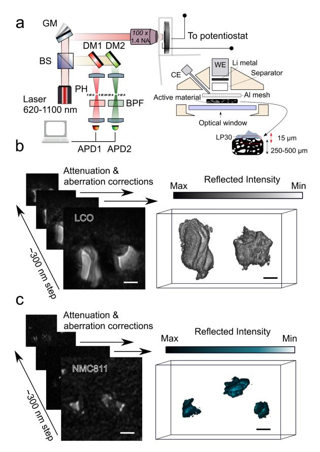
**Figure 2:** Single particle three-dimensional imaging in polycrystalline battery electrodes. a. Cartoon schematic of laser scanning confocal microscopy (LSCRM) setup and *operando* battery cell. A tunable laser source is directed to microscope body *via a* beam-splitter (BS) with reflection signal
