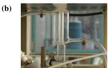
**Figure 2.** Photos of the designed bench-scale reaction units: (a) quartz tubular reactor and its furnace with upstream, the mixing/preheating unit (quartz annular exchanger surrounded by a roll of heating resistances); (b) quartz annular fast quenching system (downstream the tubular reactor).
