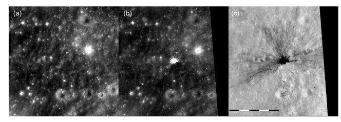
Figure 5. (A) The 'before' image, M1180620010R, taken on 2015-03-10. (B) The 'after' image, M1315871095R, taken on 2019-06-22, (C) The ratio of the two images. All three images are at the same scale of  $1.12 \text{ m pix}^{-1}$ , the scale bar is 500 m, and each segment 100 m. Cropped from PYNAPLE processed NAC images from NASA/GSFC/ASU.
