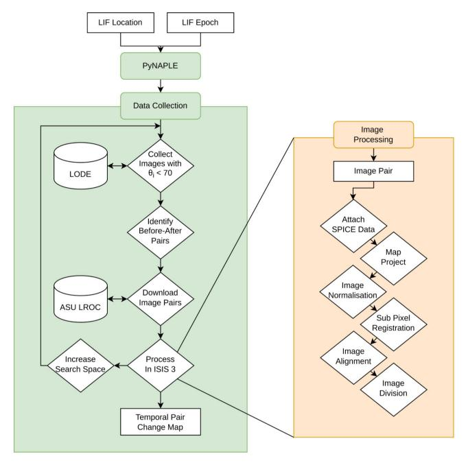
Figure 1. The PYNAPLE algorithm works in two distinct sections, data collection and image processing, and utilizes the publicly-available online LROC image repositories; the *Lunar Orbital Data Explorer*, and ASUs *LROC Image Search*, and the image processing capabilities of USGSs ISIS3. Rectangular boxes are data, diamond boxes are processes, and cylindrical boxes are online resources.
