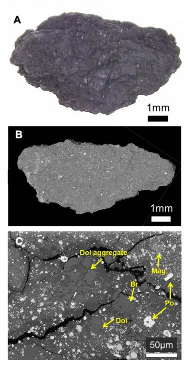
**Fig. 1. Morphology and internal texture of C0002.** (A) Optical micrograph of entire C0002 sample. (B) CT image of the largest cross section, showing the absence of chondrules and CAIs. (C) Back-scattered electron (BSE) image of typical internal texture. Dolomite (Dol), breunnerite (Br), pyrrhotite (Po), and magnetite framboids (Mag) are labelled; these are embedded in a fine-grained phyllosilicate matrix.
