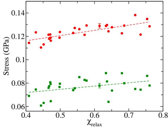
Figure 15:  $\sigma_{US}$  (red data) and  $\sigma_{25-50}$  (green data) as a function of the crystallinity degree  $\chi_{relax}$ . Dashed lines are linear regressions of each data set. Error bars are stress fluctuations and are given on a single point.
