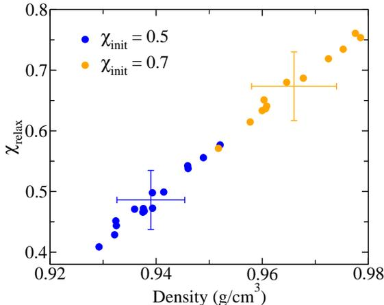
Figure 8: Crystallinity degree as a function of density for all studied structures. Blue and orange symbols correspond to structures with  $\chi_{init} = 0.5$  and  $\chi_{init} = 0.7$  respectively. The two crosses indicate the average crystallinity and average density with corresponding standard deviation.
