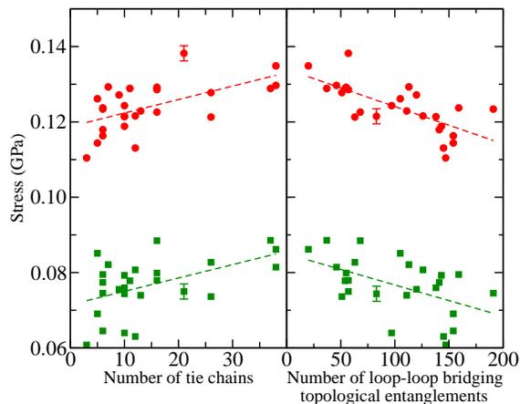
Figure 16:  $\sigma_{US}$  and  $\sigma_{25-50}$  as a function of the number of ties chains and loop-loop bridging topological entanglements. Error bars are stress fluctuations and are given on a single point.
