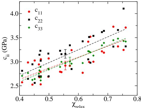
Figure 11: Tensile elastic coefficients  $c_{ii}$  as a function of the crystallinity degree  $\chi_{relax}$  of all the modeled structures. Error bars represent statistical errors and are represented once for each coefficient.
