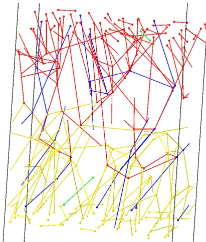
Figure 9: Primitive path of chains in an amorphous region computed with the Z1 code,<sup>56</sup> the segments belonging to loops are yellow and red, the segments belonging to tie chains are blue, the tail segments are in green. The spheres represent the primitive path kinks and the ends of the chains.
