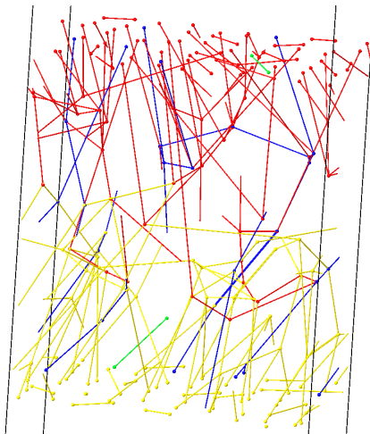
Figure 9: Primitive path of chains in an amorphous region computed with the Z1 code, 56 the segments belonging to loops are yellow and red, the segments belonging to tie chains are blue, the tail segments are in green. The spheres represent the primitive path kinks and the ends of the chains.
