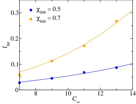
Figure 2: Fraction of tie chains,  $f_{\text{tie}}$ , as a function of the characteristic ratio  $C_\infty$  as obtained from the theory (full lines) and for the samples built in this study (symbols) for the two crystalline ratios studied here.
