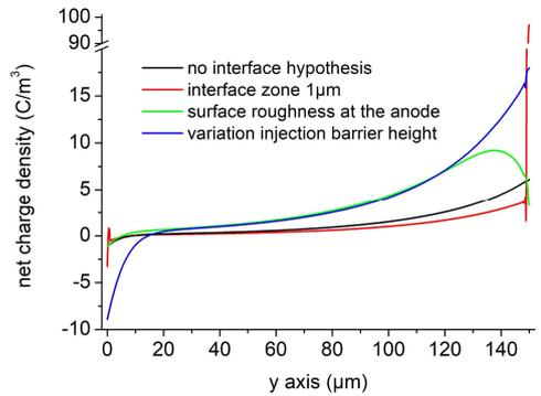
Fig. 3. Net charge density for different hypotheses on the charge generation at interfaces, compared to the case where no hypothesis is accounted for, and for  $t=300s$ . Parameters of Table I, unless otherwise stated.
