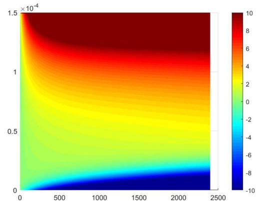
**Fig. 6.** Net charge density cartography as a function of time and depth in the sample, for a variation of the barrier height for electrons and holes of 10% around the optimized value found in Table 1.
