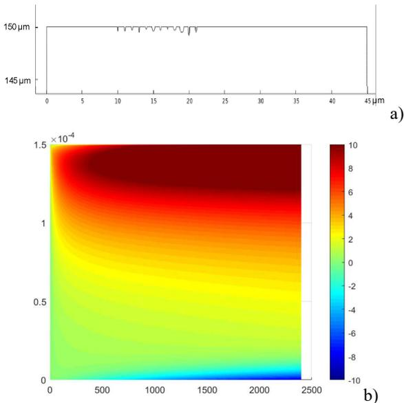
**Fig. 4.** a) Zoom of the rough zone on the top electrode surface, and b) Net charge density cartography as a function of time and depth in the sample, for a rough top electrode as proposed in Fig. 4a.
