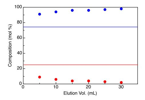
**Figure 6.** Molar fraction composition ( $C_{60}$ : blue circles;  $C_{70}$ , red circles) of fractions collected from a solution of fullerene mixture separated over an LC column packed with **1** as determined by HPLC (150 x 10 mm, eluent: toluene). The red and blue lines indicate the composition of the initial mixture in  $C_{70}$  and  $C_{60}$ , respectively.
