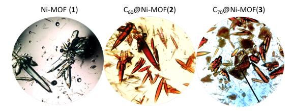
**Figure 2.** Optical microscope images of Ni-MOF (1),  $C_{60}$ @Ni-MOF (2) and  $C_{70}$ @Ni-MOF (3) at 10× magnification.
