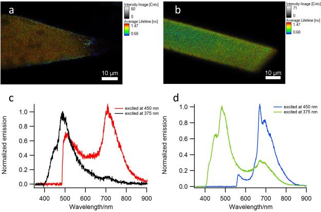
**Figure 4.** Fluorescence lifetime images from single crystals of **2** (a) and **3** (b). Emission spectra collected from single crystal of **1** with encapsulated  $C_{60}$  (c) and  $C_{70}$  (d) upon excitation of the anthracene chromophore in the MOF (at 375 nm) or of the fullerene (at 450 nm).
