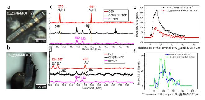
**Figure 3.** Single crystals of  $C_{60}$ @Ni-MOF (2) and  $C_{70}$ @Ni-MOF (3) (panels (a) and (b), respectively) and Raman spectra comparing the signals obtained from these crystals and those of 1 or  $C_{60}$  (c) or  $C_{70}$  (d). The intensity of the Raman signal of the encapsulated fullerene and of 1 measured along the crystal's cross-section is shown in (e) and (f) for 2 and 3, respectively (785 nm excitation laser with 5 µm steps).
