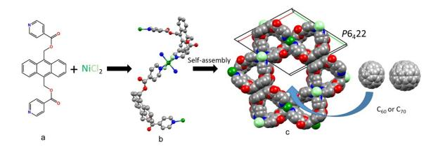
**Figure 1.** Synthesis of Ni-MOF **1** showing the conformational rearrangement of the ligand leading to the helical structure of the Ni-MOF assembly and view along the *c*-axis in the crystal structure of **1** revealing a hexagonal architecture and projection along the two types of pores with  $\emptyset$  15.6 Å and 8.1 Å. Encapsulation of fullerenes is proposed to occur in the larger pore. (Hydrogen atoms are omitted for clarity).
