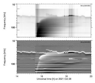
**Fig. 11.** Dynamic spectrogram at km-wavelengths observed by Wind/WAVES/TNR (*top panel*) and frequency-difference spectrum of TNR (*bottom*). Vertical bars in the top panel are artefacts, due to the spillover of intense emission in some channels to the entire receiver.
