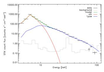
**Fig. 8.** X-ray count flux spectrum from STIX observations, at 15:27:59 UT with an integration over 0.5 s. The observed count flux is shown by the thick black crosses, the pre-flare background spectrum is shown by the thin black line, and the fitted spectrum is shown by the green line. The thermal component of the fitted model is shown in red, and the non-thermal power-law component is shown in blue.
