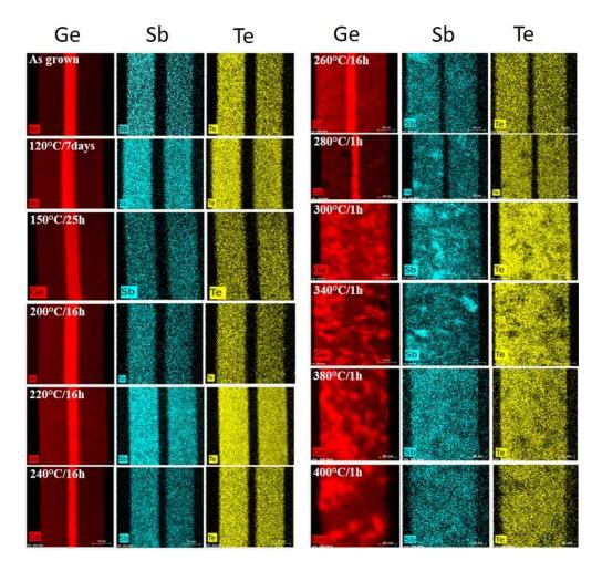
**<u>Figure 4</u>**: A series of chemical maps obtained by EDX showing the distribution of Ge, Sb and Te species in the structure after annealing. The GST-225 layers remain homogeneous up to temperatures of around 240°C.
