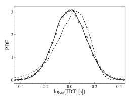
Fig. 5: Comparison of the reconstructed PDF for GRI~3.0 mechanism: —, ASM;  $\circ$ , Monte Carlo; ---, LAAM.
