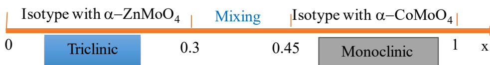
Fig.4. Structures and phase compositions of Zn 1-x Co x MoO 4 compounds.
