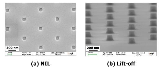
Fig. 2. (a) 100 nm patterns obtained in TU resist post NIL (b) post Ni deposition and lift off to create a hard mask.
