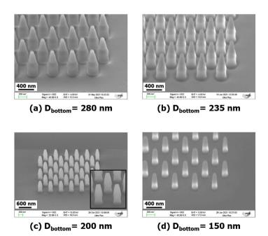
Fig. 6. Plasma chemistry effect on nanopillars profiles; (a) increase of Ar concentration ( $Cl_2/CH_4/Ar = 39/12/90$ ); (b) increase of  $Cl_2$  concentration ( $Cl_2/CH_4 = 43/8$ ), (c) pure  $Cl_2$  (80 sccm); (d) pure  $Cl_2$  (80 sccm) on an Oxford Plasmalab 133 reactor with a chuck cooled down to 5 °C.
