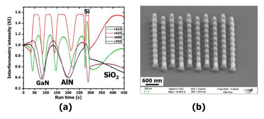
Fig. 3. (a) Real-time etch control is monitored using optical interferometry and (b) a 100 nm pillar array without any defect.
