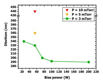
**Fig. 5.** Plasma parameter modification: three different etching pressures and bias power VS Dbottom for the same Dtop of 100 nm.
