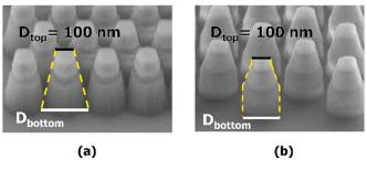
Fig. 4. Optimization of SiO2 sidewalls.
