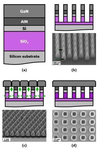
**Fig. 1.** Technology developments: (a) GaN on SOI stack, (b) nano-pedestals generated post lithography and etch, (c) GaN step 1 growth: selective nucleation and the principle of  $SiO_2$  pillar twist during GaN epitaxy, (d) GaN step 2 growth: lateral growth. Each GaN mesa is grown on arrays of pillars/pyramids as those in (b) and (c).
