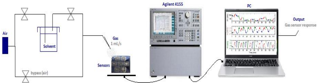
102 103 Fig. 1 E-nose setup used for measuring the resistance of gas sensor
